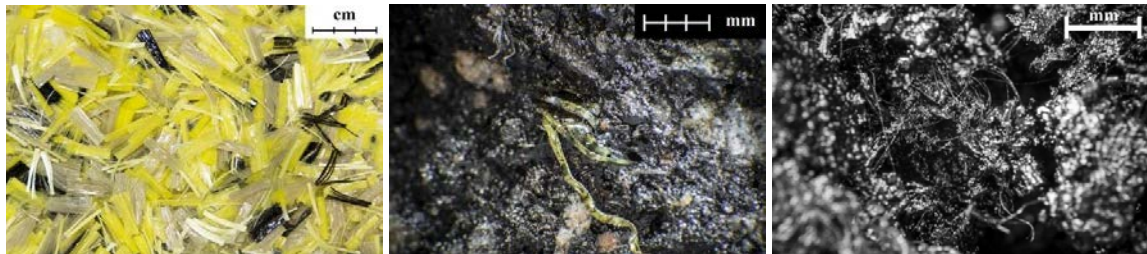
Fig. 1. a) Loose fibres, b) Fibres in laboratory mixed asphalt concrete, c) Fibres in plant mixed asphalt concrete, (all photos by Ł.Mejłun).
